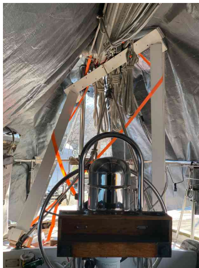
Photo 1: The first mast support failure. After the second failure, the 300-lb. mast dropped all the way to the pushpit rail.
